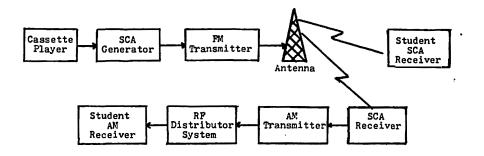
Figure 1. Block Diagram of the Subsidiary Communications Authorization (SCA) Transmission and Reception Process.
