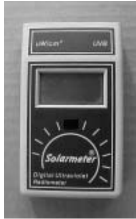
The low-cost hand-held ultraviolet radiometer from Solarmeter (model 6.2) provides hobbyists with the ability to take their own UV-B readings.
