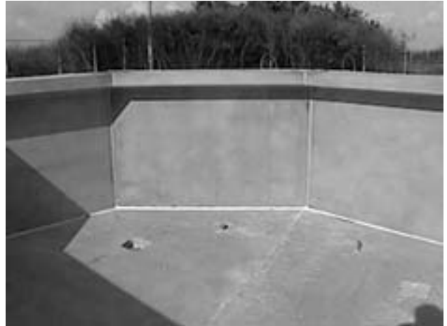
Small-scale test arenas, such as this concrete model built at the Guam NWR, were the final testing stage for all of the snake barriers we developed.
