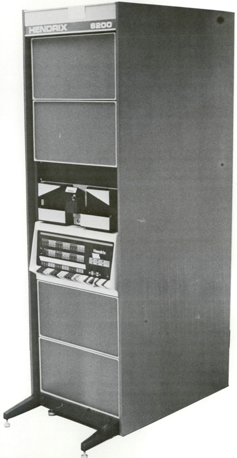
The Hendrix 6200 controller stores the copy that is fed into it from the scanner and retrieves it for editing on the video display terminals.
