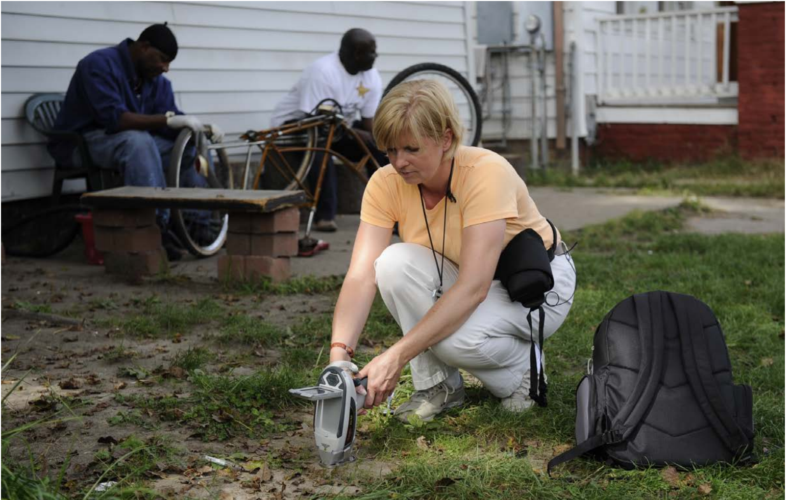
As an investigative reporter for USA Today, Alison Young spent weeks on the road testing soil with a handheld X-ray device in neighborhoods around long-closed lead smelters as part of her Ghost Factories investigation. (Photo courtesy of USA Today)
