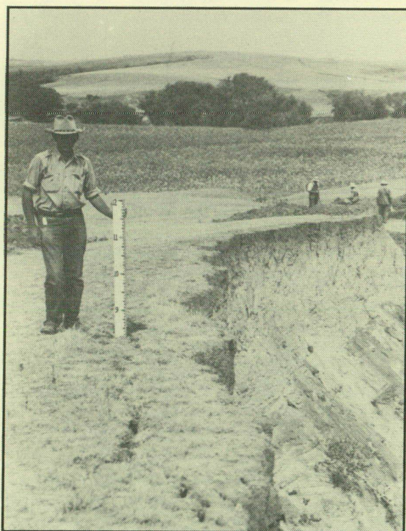
Carlyle Shreve Smith measuring depth of crack in bluff above Davis Creek at site GY-4, Nebraska, 1941.
