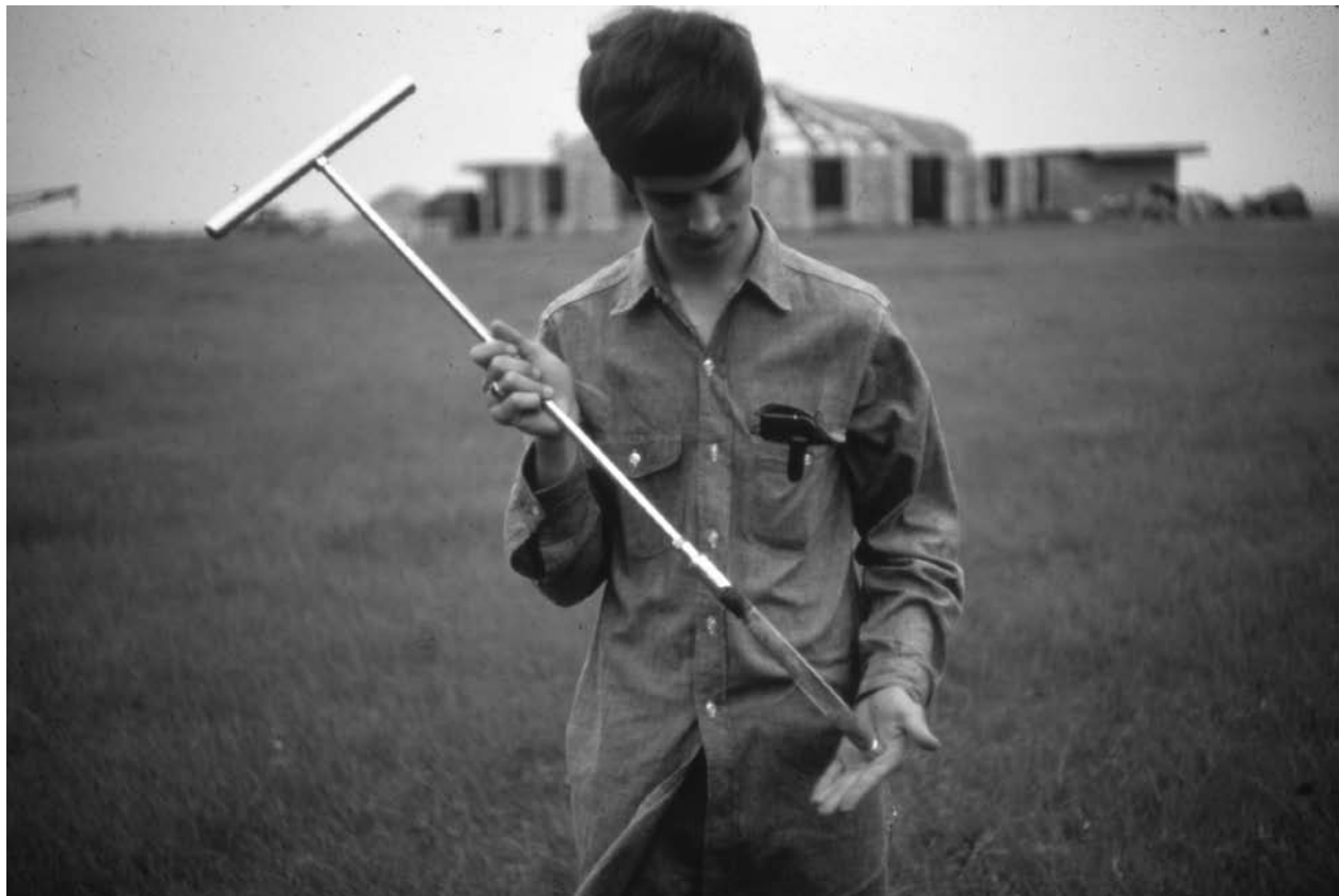
Figure 2. Oakfield soil sampling tool, displaying subsurface soil strata.
