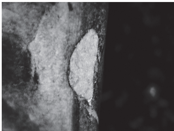
Figure 57. Type C: Indicative of another deeper and broader mechanism, this type of extractor mark is typical of falling block rifles, such as the various Sharps models.
