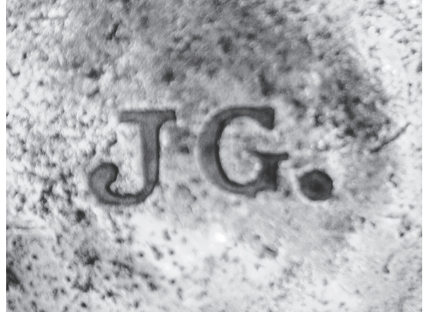
Figure 63. Usually found on the Spencer .56–50 cartridge, the J.G. headstamp indicates a Joseph Goldmark manufacture during the post-Civil War and Indian Wars eras.
