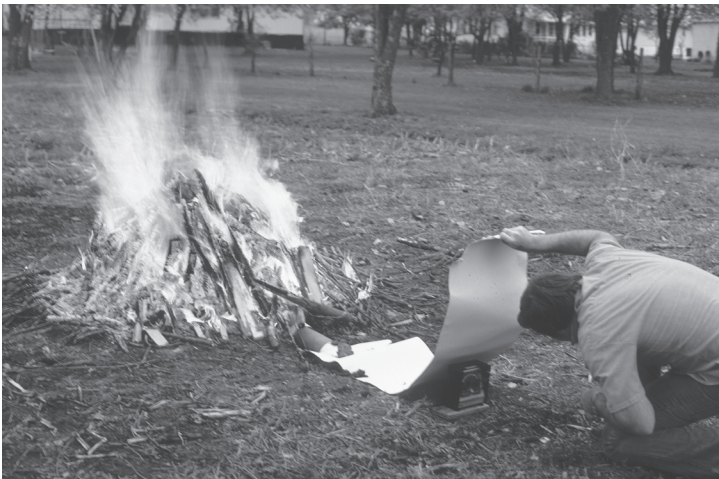
Figure 2. Taking a pyrometer reading during firing from behind a protective asbestos sheet.
