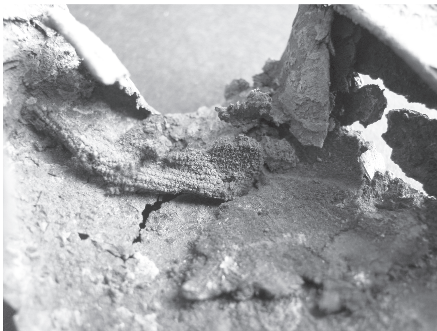
Figure 11. Detail revealing lack of wear on underside of case's cloth liner center section.
