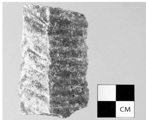
Figure 22. Structural or foundational stone corner fragment with chisel marks in a herringbone pattern. Courtesy of Kansas Memory, Kansas Historical Society, Topeka.
