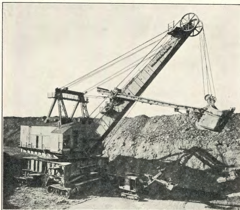
PLATE 9. A, View of an area of about 600 acres that has been stripped for the Bevier coal. The coal is about 20 inches thick. View looking south from near the center of south line sec. 9, T. 28 S., R. 25 E.; B, Type of electric shovel used in removing overburden from the coal in the southeastern Kansas coal field. Note ordinary steam shovel below boom.
