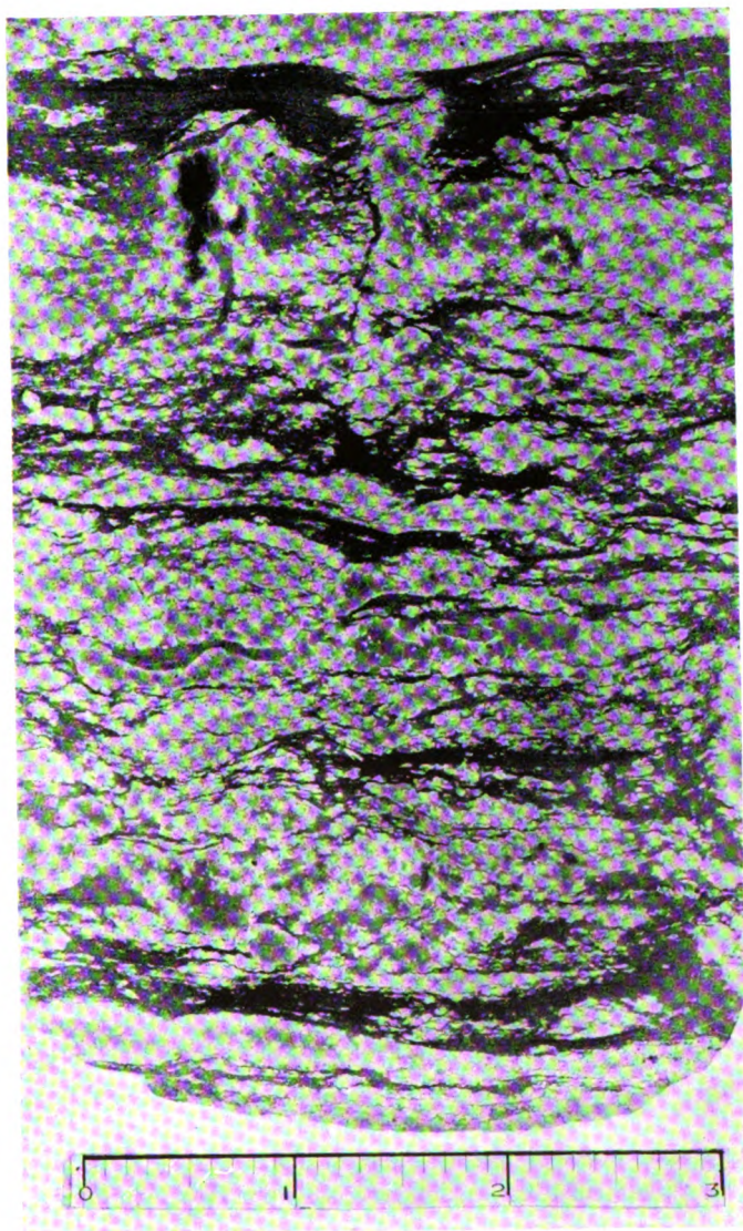
PLATE 9.—Photograph of polished section of core from upper part of Cowley formation in Patton Drilling Company No. 1 Rogers well, in sec. 35, T. 31 S., R. 2 W., Sumner county, Kansas. The photograph shows the laminated character of the silty limestone. In this core the Cowley contains a much larger proportion of chert (shown by the lighter areas) than is usual. The laminae are shown to be interrupted by the chert. Both the chert and siltstone are crowded with spicules and the remains of calcareous microörganisms. Photograph is natural size.
