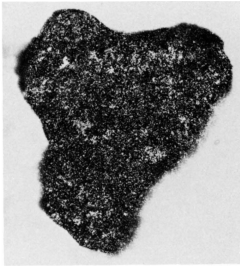
Figure 5. Radioluxograph of silicified Ogallala Formation (sample U-6, 123 ppm U_3O_8 , exposure time 70 hours) shows the fairly even distribution of radioactive material throughout the sample. Radioluxograph made by J. R. Dooley, U.S. Geological Survey, Denver.
