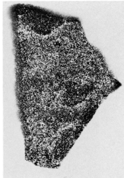
Figure 6. Radioluxograph of silicified Ogallala Formation (sample U-2, 62 ppm U_3O_8 , exposure time 144 hours). Partially silicified and less radioactive clasts are easily identified. Radioluxograph made by J.R. Dooley, U.S. Geological Survey, Denver.
