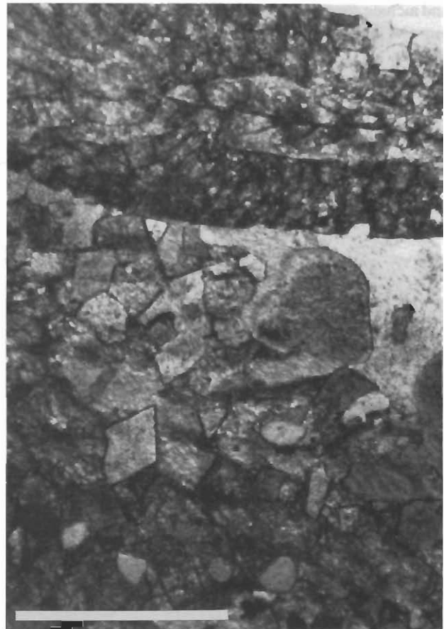
FIGURE 16—PHOTOMICROGRAPH OF LIMESTONE FROM UNIT D showing bryozoan and echinoderm fragments. Sample EB6347 from Sinclair–Prairie No. 1 Exchange Bank, sec. 27, T. 33 S., R. 19 W., Comanche County, Kansas. The bar scale is 1 mm.
