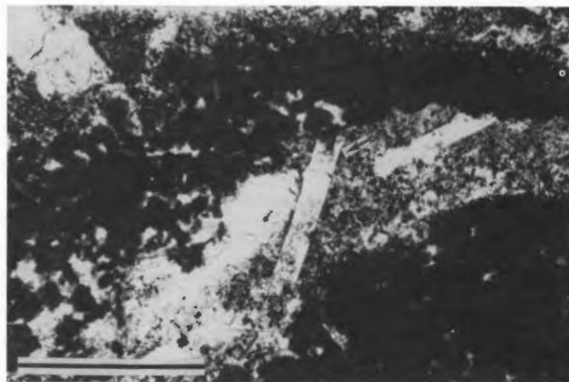
FIGURE 11—PHOTOMICROGRAPH AT HIGHER MAGNIFICATION OF THE SAME PSEUDOMORPHS of evaporites shown in fig. 10. Scale bar is 1 mm.
