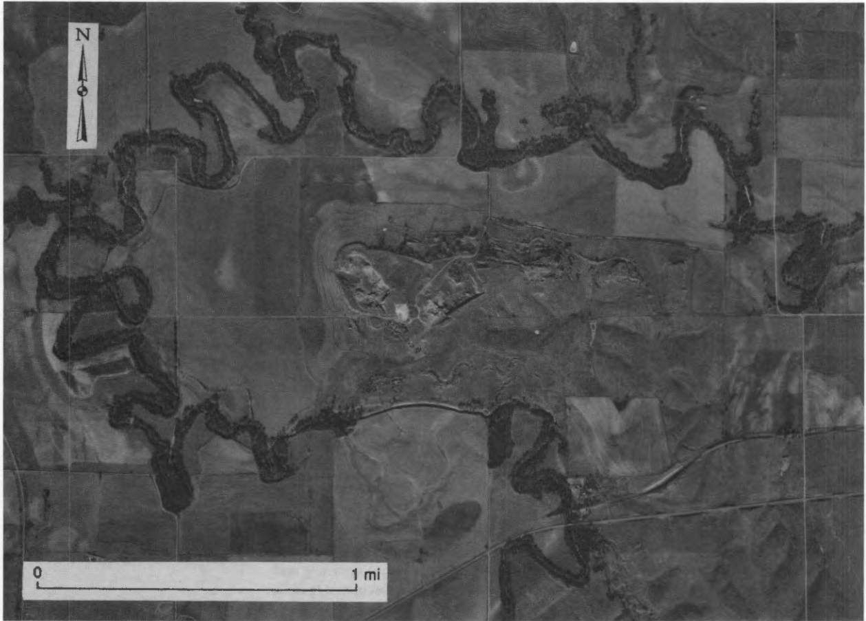
FIGURE 15—The anomalous westward deflection of northeastward-flowing Prairie Dog Creek around a ridge capped by a silica-cemented sandstone bed in the Ogallala Formation. The quarries from which the silica-cemented sandstone has been extracted are apparent on the west end of the ridge. The railroad cut in the lower right sector exposes sand and gravel of Illinoian age overlain by the Gilman Canyon and Peoria formations (loesses).
