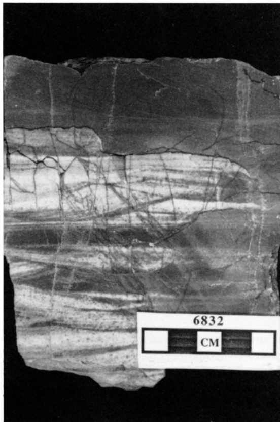
FIGURE 7—PELOID GRAINSTONE/PACKSTONE FACIES FROM THE HUGOTON MEMBER IN THE MOBIL #1 FOSTER. Ripple cross laminations highlighted by chert. 6,832 ft core depth.
