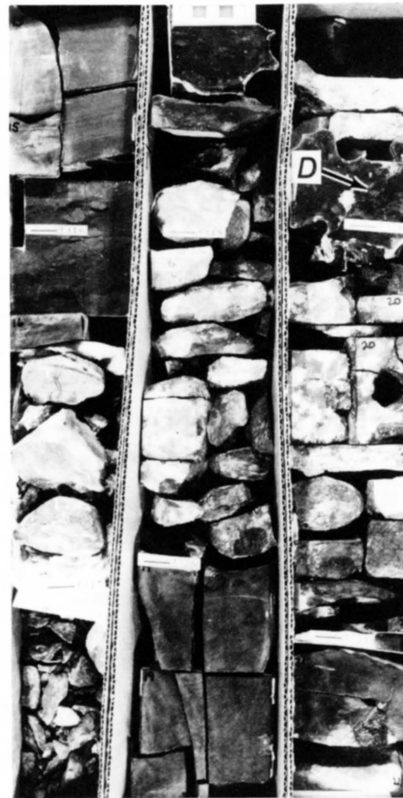
FIGURE 8—MAROON CALCAREOUS SHALE (5,316.8–5,319.0 ft [1,595–1,596 m] and 5,319.5–5,320.2 ft [1,596 m]) INTERBEDDED WITH PELOID PACKSTONE. Light patches (just above 5,320 ft [1,596 m]) are interpreted as drab-haloed root traces (D) formed by the reduction of iron during anaerobic decay. 5,315–5,321-ft (1,594–1,596-m) core depth, Amoco #1 Breeding F.
