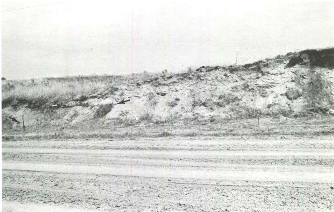
FIGURE 20. Exposure of cemented alluvial sand and gravel, tentatively assigned to the Ogallala Formation, in the uplands of the SE sec. 9, T. 11 S., R. 15 W. In this roadcut, the Ogallala unconformably overlies the Blue Hill Shale Member of the Carlile Shale (arrow).
