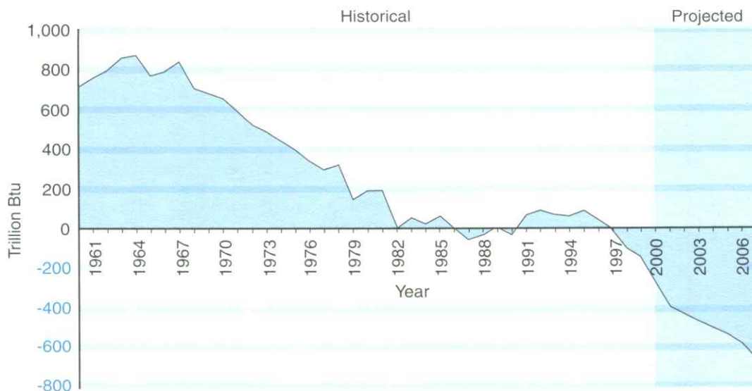
Figure 13—Kansas Net Energy Balance, 1960–1999, with Projections to 2007. Positive numbers show energy produced in excess of consumption (exports), while negative numbers show energy consumed in excess of production (imports). Sources: Production data (see Tables 1, 2); consumption data (see Tables 6, 7); projected production and consumption (Carr, 2002a; SERCC, 2003).
