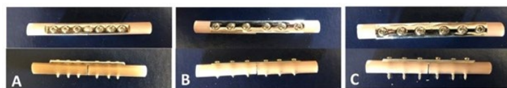
Figure 1. Plate constructs used in this study included: (A) 2.7-mm LC-DCP plate, (B) 1/3 tubular plate, and (C) stacked 1/3 tubular plates.
