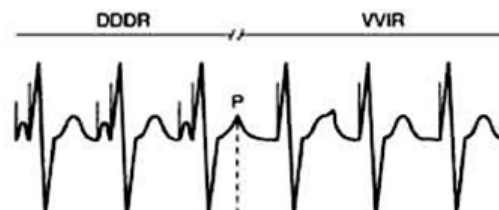
Figure 1. Schematic illustration of EMI-induced conversion to VVI pacing from DDDR pacing mode after electromagnetic interference.
