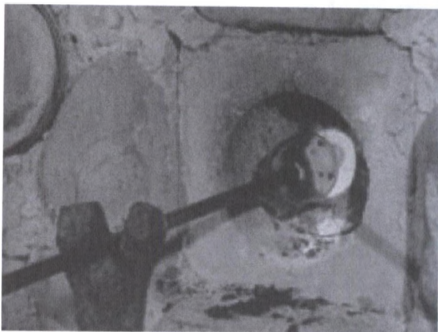
Fig. 7. Glory hole in glass oven of a simulated Glasshouse at Jamestown, VA. The glassblower inserts his blowpipe into the furnace to re-heat the glass bubble at its end. Courtesy of U.S. National Park Service.
